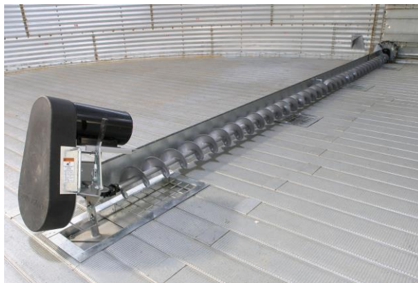
Figure 15: Silo Sweep Auger
