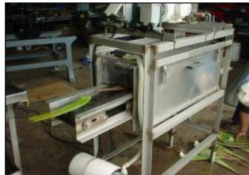
other foreign material from the surface of the leaves. Depending on the capacity of the plant one or several simultaneous lines of brushes can be installed. Usually the material of choice for these brushes is soft plastic, which vigorously removes unwanted material from the surface of leaves while being gentle enough to prevent injury to the leaf.
