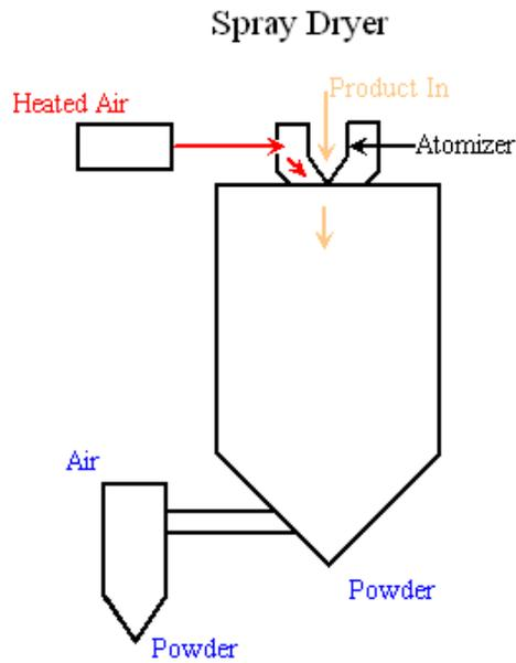
Spray dryers work by converting the Aloe concentrate into a very fine mist of droplets. The droplets form in a conical shaped chamber when the concentrate encounters flow of warm dry air. This then causes the drops to become so small that it increases the surface to volume ratio of the drop facilitating evaporation. The droplets are suspended inside the chamber until they become denser due to the evaporation. They then fall to the bottom of the chamber in a powder form and collected.
