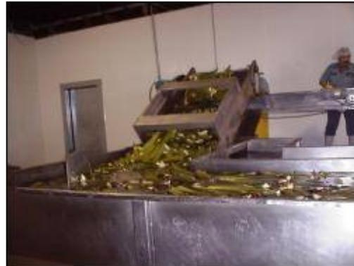
b. Forced agitation: This is a variation in which the tank has high pressure water jets that create a whirlpool in the soaking tank. The advantage of using this system is that dirt and other foreign material is removed in a more efficient way.
