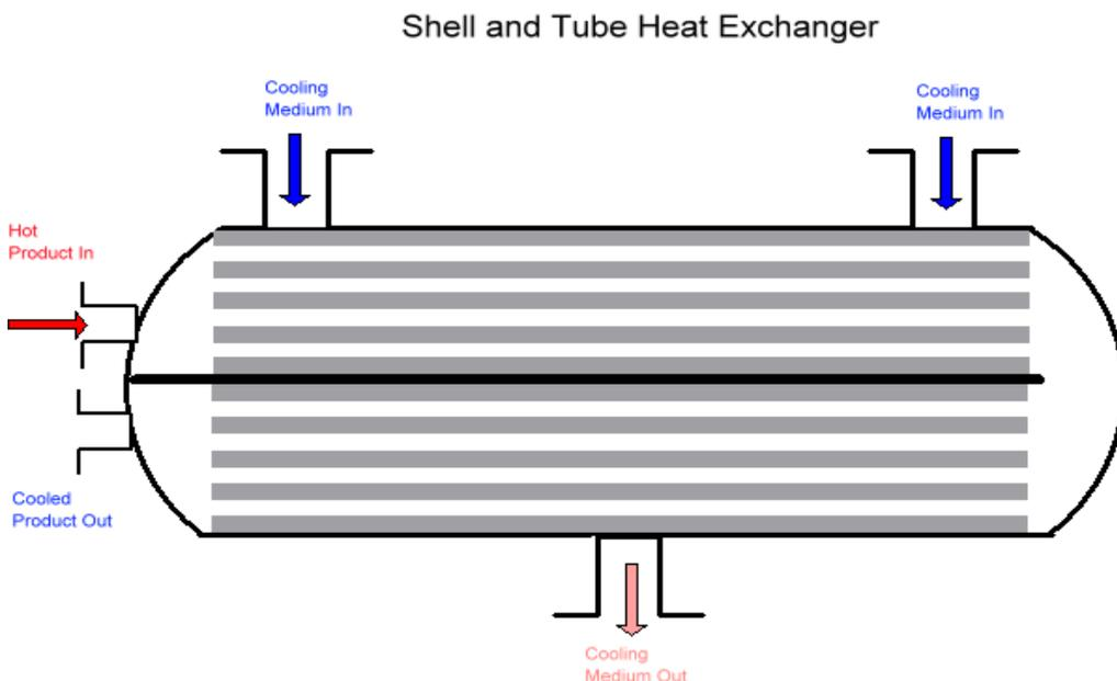
Shell and tube heat exchangers consist of a bundle of parallel sanitary tubes with the ends expanded in tube sheets. The bundle is contained in a cylindrical shell. Connections are
